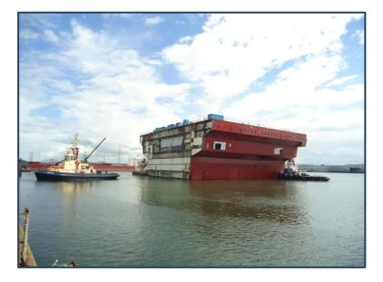
And finally, with both blocks in place, the dock was drained and both blocks docked down.
