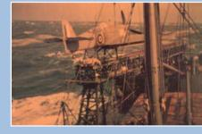
The major draw back of CAM ships, however, was that once the pilots had completed their mission they had to bale out or ditch in the sea and rely on being picked up by one of the ships. The first pilot to successfully launch from such
