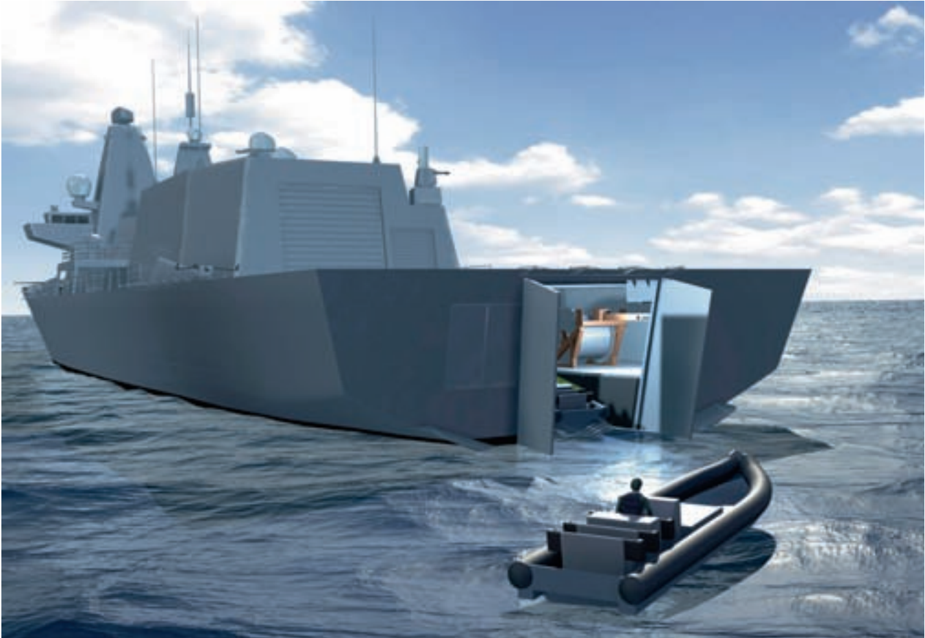
The general-purpose version of the Type 26 frigate will launch boats from the stern instead of over the side
